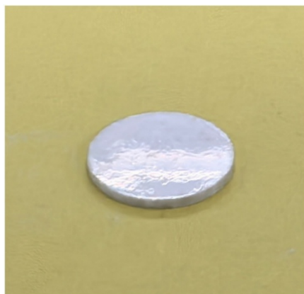
Supplementary Figure 3. The ZHP pellet is approximately ~1 mm thick and 10 mm in diameter by pressing ~200 mg of the powder of ZHP at 407 MPa.
